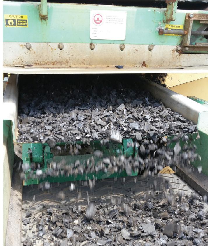
To produce TDF, tires are first shredded, ground and screened into small chips. For some applications, steel is retained. For others, a smaller, low-steel-content tire chip is more appropriate.
