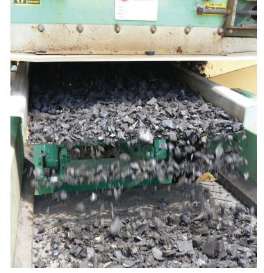
To produce TDF, tires are first shredded, ground and screened into small chips. For some applications, steel is retained. For others, a smaller, low-steel-content tire chip is more appropriate.
