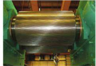
Granutech's new G-4X Mill is designed to process scrap rubber, featuring sealed roller bearings for greater tolerances when processing in as small as 80-mesh.
