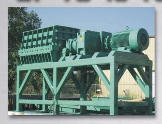
The SATURN GRIZZLY™ SUPER 80 (S-80) by Granutech-Saturn Systems is a next-generation, high performance secondary grinder. The S-80 provides the highest throughput in a single machine for tire recycling with an output up to 200 tons per day.
