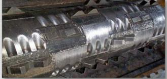
The SATURN GRIZZLY™ Super 50 (S-50) is a medium speed grinder that excels at reducing tire shreds into near steel free chips. The rotor knife arrangement contributes to the extremely efficient cutting action and high production capacity. The S-50 is designed for low capacity requirements. A multi-use knife design contributes to the S-50's low costs of operation.
