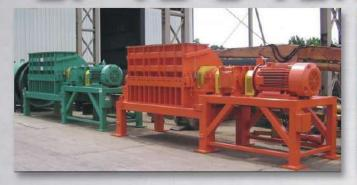
For nearly two decades, the SATURN GRIZZLYTM Model 80 (M-80) has excelled at reducing tire shreds to virtually steel free chips. The massive rotor, low cost knife design, and replaceable screens provide a highly reliable and efficient operation process. Due to the knife design, product from the Model 80 Grizzly is ideal for playgrounds and landscaping.
